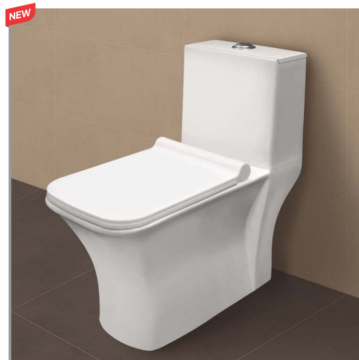
Nexo Code 1130 L 685 W 360 H 705mm / L 27" W 14.15" H 27.75" Siphonic S-trap Central of outlet 90mm & Wall distance 240mm (9")
