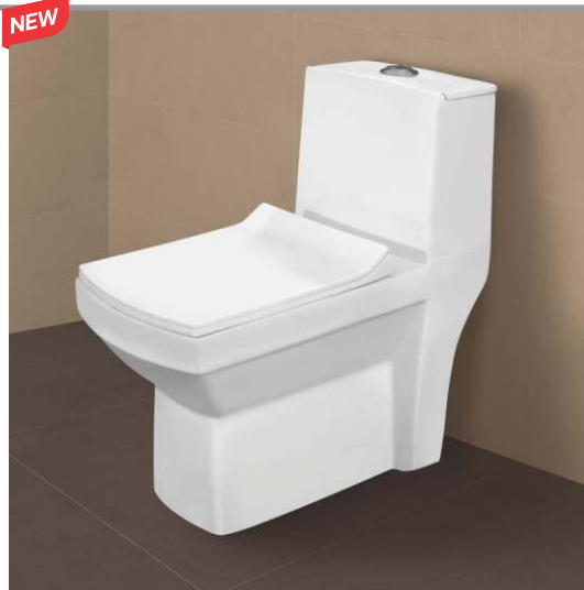
Tango Code 1146 L 690 W 345 H 705mm / L 27" W 13.5" H 28" Wash Down S-trap Central of outlet 90mm & Wall distance 100mm (4")
